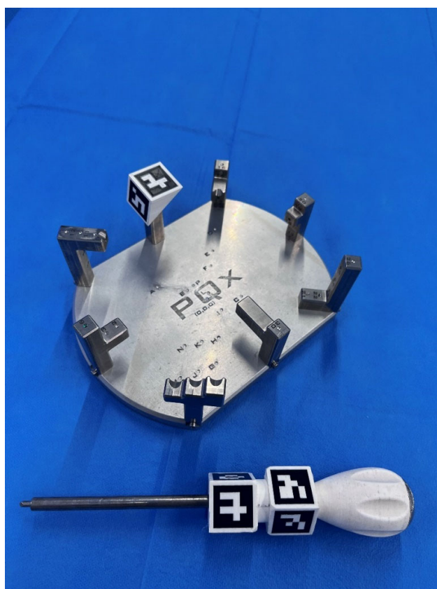
Figure 1. 316 L steel model used for distance and angle measurements and stylus. Both have ArUco-type artificial markers. The relationship between the palpation points has been arranged with different levels of access difficulty for both right-handed and left-handed observers.
