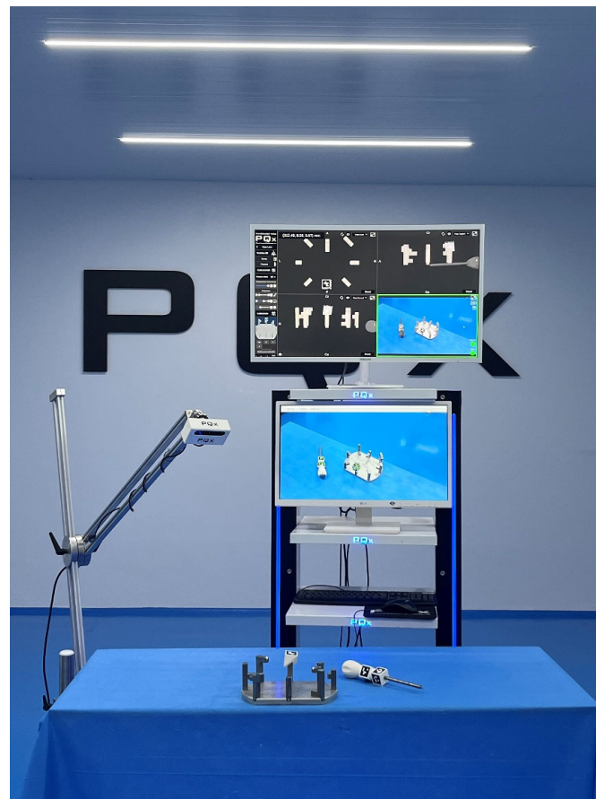
Figure 3. Devices used in the experiment: platform with palpation towers, optical camera, central processing unit and monitors. The monitors were positioned centrally in front of the observers so that the exchange of information between the real, virtual and AR domains could occur with a simple eye-raising gesture.
